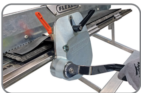
Single Blade Belt Skiver skives belts up to 50 mm thick. Maximum skive per pass is 10 mm.
