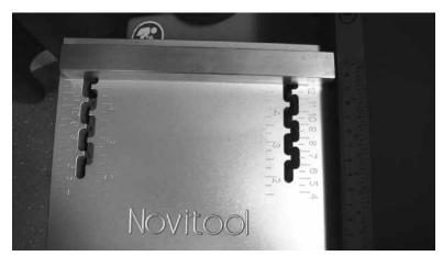
Lock adjusting guide to 120 mm.
