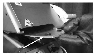
Insert nuts so that bevels are facing toward traction rollers.
