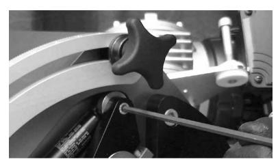
For upper roller adjustment loosen and remove gas spring fixation screw.
