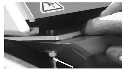
Tighten bolts firmly while keeping pressure of blade against the jig.
