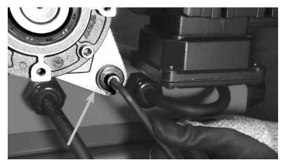
Remove the electric motor to gain sufficient access for adjustment of traction rollers by first removing the torque arm bolt using a 6 mm hex wrench.
