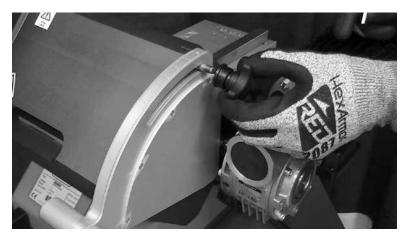
If adjustment is needed, unscrew clamp nut on adjustment guard plate.
