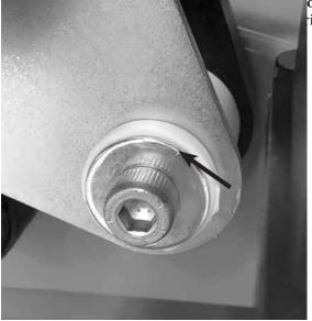
**ote:** Ensure rubber grommet is in place rior to reassembly.
