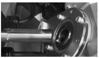
Reinstall motor. Align shaft key with key slot.
