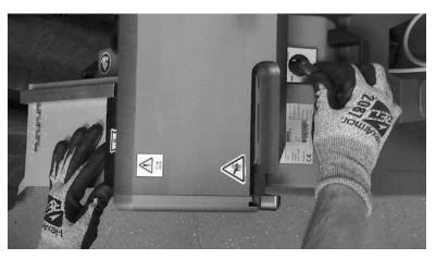
Reconnect power cable to electrical power supply. Rotate switch to 'REVERSE' to release calibration jig from between traction rollers.
