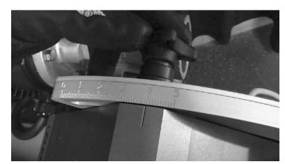
Lock adjusting handle in position 4.0 to 4.5.
