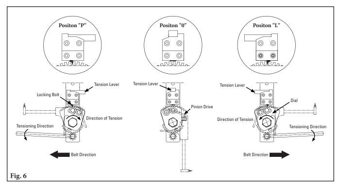
Position "P"- Right Tension: direction of tension is towards the right (clockwise) only.
