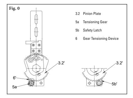
The HD tensioning device differs from the standard tensioner with the construction of the pinion plate (Fig. 0-3.2) and the safety latch (Fig. 0-5b). The HD tensioning device is recommended for use in applications with belt widths greater than 1200 mm. This solution is used for lighter tensioning of the cleaner, allowing for a larger gear ratio (Fig. 0-6).
