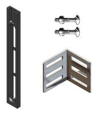
1. Assemble the back plate to the triple slot angle bracket using two carriage bolts.
