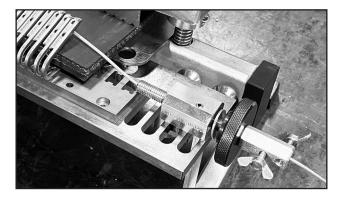
2. Position End Block approximately 2 H-holes from left edge of the belt. Insert XP-LOK<sup>TM</sup> Belt Wire through blocks on both ends of the bed between belt and fastener. Leave minimum of 50 mm (2 inches) of excess wire on each end.
