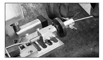
**3.** <u>Hand tighten</u> 2 wing screws on End Block (M5 thread). Pull wire taut on Tensioning Block end and ensure wire is located between fastener holes. <u>Hand tighten</u> remaining 2 wing screws.
