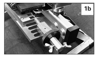
**1.** Load XP<sup>™</sup> Staple Fasteners in the bed starting on the right side. Leave 2-3 empty H-holes. Center belt in fasteners and tighten clamp bar. Insert Tensioning Block into the last slot of the bed. Fig 1a. Ensure Tensioning Knob is in the out position by pulling the threaded shaft all the way out. Rotate the Tensioning Block 90 degrees to the right to lock into position. Fig. 1b.
