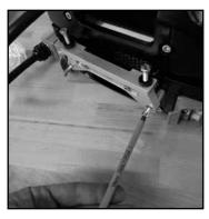
**Step 4**. With 5mm hex wrench tighten bolts firmly in place.
