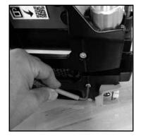
**Step 1.** On bottom press beam end plate with a 5mm hex wrench, remove the top bolt on both sides and discard.
