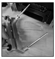
Step 2. From End Belt Clamp Kit, install two long bolts into one end clamp assembly. The bolt head will seat in the countersunk indentation. Place one spacer over each bolt.
