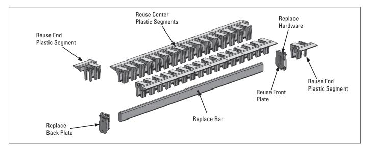
2. Replace the indicated items with the new stainless steel components. All metal components of the STP (with the exception of the front plate) must be replaced with stainless steel parts. This includes the support bar, end plates and hardware (fasteners, washers, shims).
