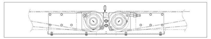
5. Install the transfer plate and follow steps 1 to 14 of IOM X4064. Once STP has been adjusted to proper height; tighten the fasteners until the washers are compressed and plus  $\frac{1}{4}$  to  $\frac{1}{2}$  a turn.
