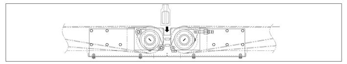
3. Insert the backplate between the pulleys and align the vertical slots with the horizontal conveyor slots. Make sure you have complete overlap between slots. You will need enough overlap to install a minimum of two fasteners. The plate must be aligned towards the feeding conveyor.
