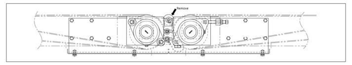
2. Remove the pop up roller and all its supporting structure including the safety cable.
