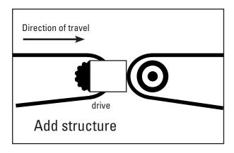
• In the particular case of waterfall conveyor arrangements (incline or decline configurations) there may be gaps where the conveyors meet. Make sure there is adequate structure to mount the transfer plate mounting brackets at the point of installation. If necessary, add a support plate to ensure safe and proper installation of the Segmented Transfer Plate mounting brackets.
