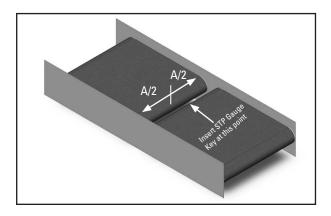
When inserting the STP gauge key, you should have a minimum distance between the top of the STP profile and the tangent point of the belt and the pulley of no less than 12.5 mm (½") in smaller diameter pulleys. For large diameter pulleys, the distance should not exceed 38 mm (1.5"). The bottom corner of the transfer plate plastic segment should have full contact with the belt and the key should rest level to the imaginary line that joins the crowns of the pulleys.
