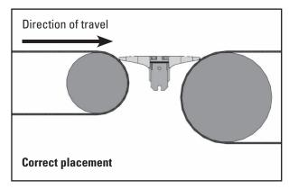
**Correct STP placement:** This is an example of a correct installation. The transfer plate is installed properly with adequate contact between the belt and the STP plastic segments.
