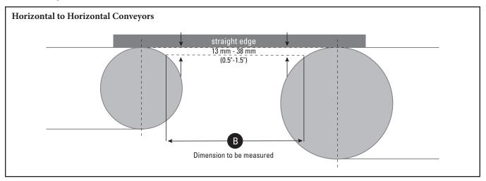
Dimension "B" will be obtained by locating a straight edge between the center lines of the pulleys. The dimension will be obtained by offsetting a parallel line towards the center of the pulley. The total offset should be between 1/2" (13 mm) to 1.5" (38 mm) below a line between the tangent points on the pulleys for most applications. The "B" dimension should be obtained by measuring the distance between the pulleys where the offset line intersects the outside diameter of the pulleys.
