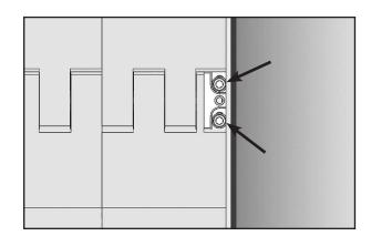
**14.** Once all adjustments are made, secure the screws on both sides of Segmented Transfer Plate assembly with a thread locking agent.
