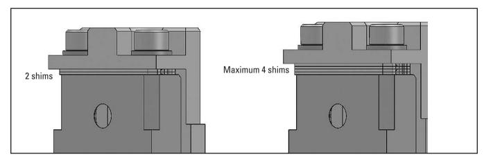
**13.** By adding or removing shims from the mounting brackets, the transfer can be adjusted up or down a total of 3 mm (1/8th inch). This should allow adequate adjustment for crowned pulleys or a belt with a profiled top cover.
