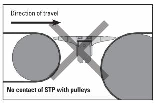
**WARNING:** This is an example of an incorrect installation. The transfer plate has no contact between the pulley and the plastic STP segments. Thin flat items and polybags will get caught in the gap and interfere with flow of material.
