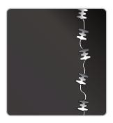
For quick temporary repairs, hammer-applied Turtle (TM) No.16 fasteners are recommended every 101 to 152 mm (4-6 inches) along the rip.
