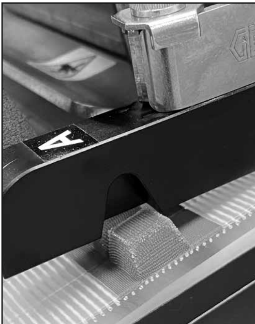
Step 9c Belt Clamped into Last V-Guide Notch
