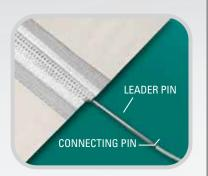
Connecting pin installation can be difficult, given both the small diameter of the pin and the flexibility of the material. To ease and speed this process we offer Leader Pins, which attach a smaller diameter, rigid lead pin to the larger diameter, flexible connecting pin. The lead pin is easily fed through the splice, allowing the actual connecting pin to be pulled through. The use of Leader Pins often reduces pin insertion time by more than 75%.
