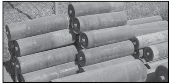
How an operation stores rollers has a big impact on corrosion. Any roller will “breathe” and wide variations in hot and cold temperatures can affect roller performance. Steel rollers, like the ones pictured above, can corrode when stored outside.
