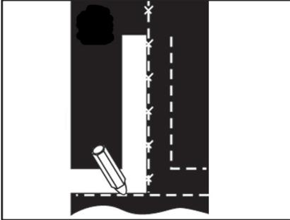
1. Square belt using centerline method. Cut belt 4" (100 mm) behind old splice using a Flexco belt cutting tool. Skive belt when top cover permits.
