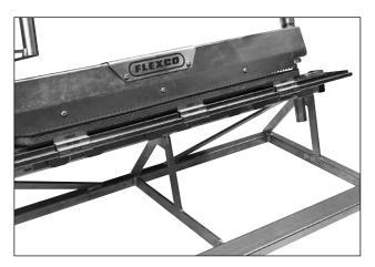
1. Select belt stops that correspond to the fastener size. Slide belt stops onto bed, evenly spaced for full belt width. Insert belt end into frame centered on the bed and until it rests against all belt stops. Tighten clamp bar.
