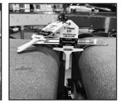
**b.** Measure the gap at the beginning, center, and end of the conveyor rollers using the FLEXCO STP gauge tool (kit item code 56707).
