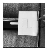
**16.** In some cases the bracket will be hidden under the metal guard of the power turn. if this is the case, make sure you have enough room to remove the fasteners so you can adjust the transfer plate.
