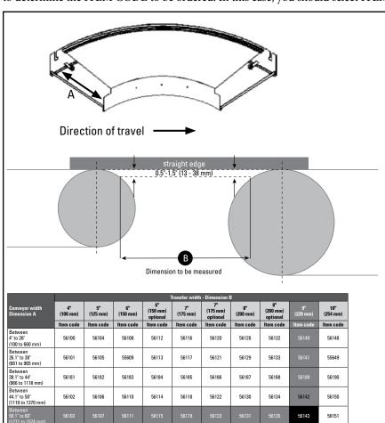
**NOTE**: Power curves operate conical rollers in both ends of the conveyor. The geometric nature of the roller will allow you to have a flat horizontal surface that will transition into a tapered vertical surface.
