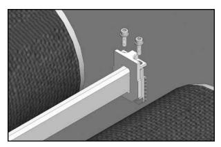
**8.** After verification that the tack weld has occurred, remove the socket head screws from the mounting brackets and lift the assembly with the front plates out of the transfer, leaving only the back plates in place and finish welding the back plates with a 1" (25 mm) bead on two sides of the plate.
