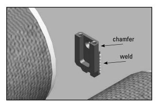
7. Welding instructions: With the assembly in place, tack weld the back plate onto the structure. Verify location after tack weld and adjust as needed.
