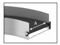
**a.** Measure the inside of the conveyor belt system.
