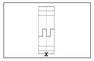
**CAUTION:** Do not trim more than half off a segment pair or 1-1/2" (38 mm). It is recommended to trim both segments of a segment pair while they are nested to ensure consistent segment.
