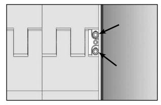
**15.** Once all adjustments are made, secure the screws on both sides of the Segmented Transfer Plate assembly with a thread locking agent.
