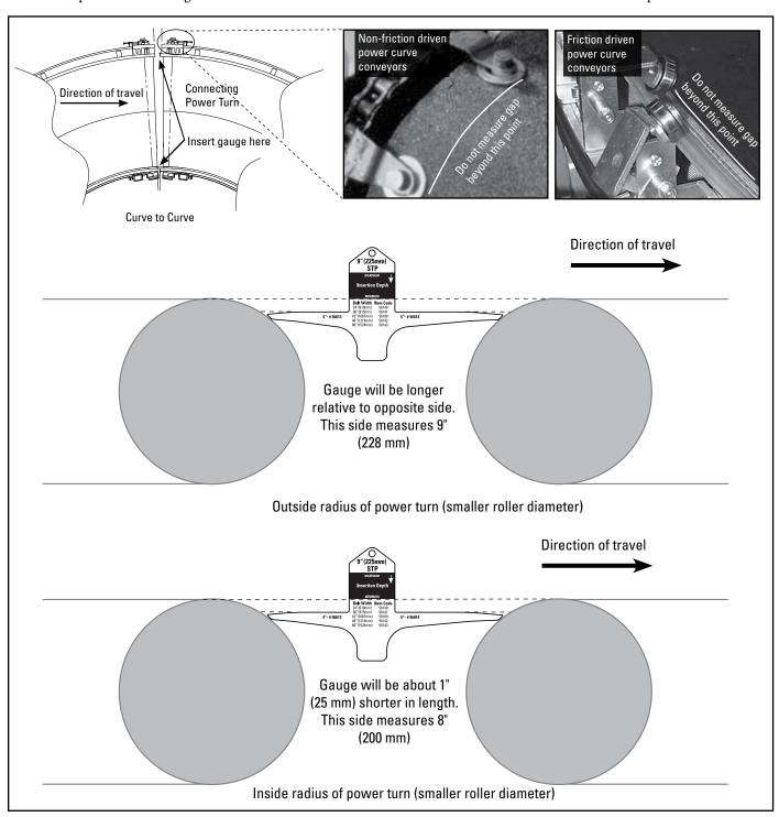
In this case, we will select the larger size 56143 STP. This will allow us to install correctly on the wider side of the transfer and adjust the opposite side by either elevating the transfer and positioning it slightly closer to the crown of the roller or cutting the plastic segments on the discharge side of the installation.
