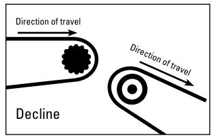
**3. Horizontal to Decline Conveyors** Both conveyors are aligned and the belts have the same direction of travel. The first belt will feed the second belt. The second belt will have a downward direction.
