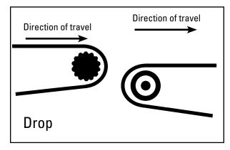
**4. Horizontal to Horizontal Drop Conveyors** Both conveyors are aligned, but not level, and the belts have the same direction of travel. The first belt will feed the second belt. There is a clear drop between the belts.
