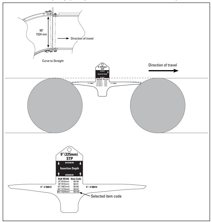
In the case of misaligned conveyors, you will have to measure the transfer gap at two locations. The locations will be the same regardless of if the gap is located between two power curves or power curve to a straight conveyor. It is imperative that the measurement is done with accuracy and ensuring proper gauge placement to avoid a product selection or installation problem.
