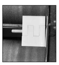
**16.** In some cases the bracket will be hidden under the metal guard of the power turn. if this is the case, make sure you have enough room to remove the fasteners so you can adjust the transfer plate.
