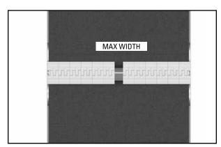
12. From the center of the bar, push the segment pairs toward the ends of the bar, ensuring that they are tightly butted against each other. Measure the gap that remains between the center-most segments to determine the size of the final segment set.
