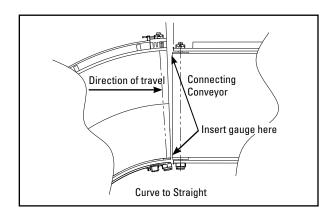
Obtaining the two measurements is necessary to determine if the transfer will cover the full gap. In some cases, a straight transfer plate will be able to cover the full gap without the need for modifications. However, in specific instances where the misalignment occurs on both the horizontal and vertical plane, you will have to account for the potential to modify the transfer plate.
