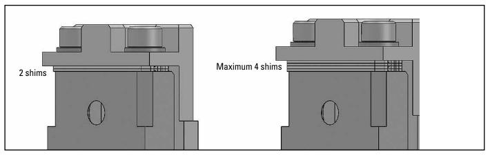
**14.** By adding or removing shims from the mounting brackets, the transfer can be adjusted up or down a total of 1/8" (3 mm). This should allow adequate adjustment for crowned pulleys or a belt with a profiled top cover.
