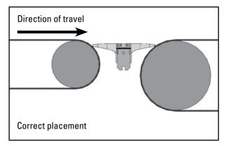
**Correct STP placement:** This is an example of a correct installation. The transfer plate is installed properly with adequate contact between the belt and the STP plastic segments.
