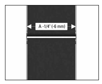
**2.** After Dimension A is determined, subtract 1/4" (6 mm) from Dimension A. The resulting measurement will be the correct size of the mounting bar holding the plastic segments.
