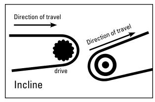
**2. Horizontal to Incline Conveyors** Both conveyors are aligned and the belts have the same direction of travel. The first belt will feed the second belt. The second belt will have an upward direction.
