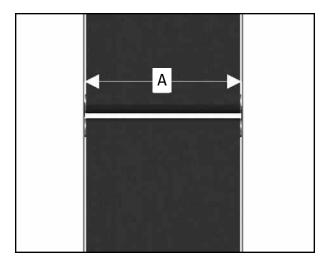
1. Measure the inside of the structure in order to determine the length of the transfer plate (Dimension A) at the point of the desired installation. This measurement will be required to properly select the transfer plate and adequately install the plastic segments of the transfer plate.
