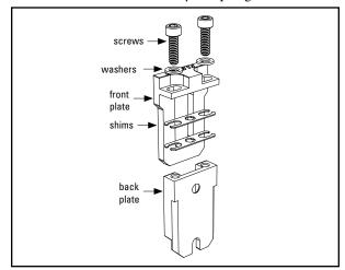
3. Stack two shims on top of back plate of each mounting bracket. Using socket head screws and washers, attach front plate to the back plate, ensuring that the shims are in place. Align the edges of the front and back plates so that the vertical edges are parallel. Tighten screws to compress shims, ensuring no interference with the pole end.
