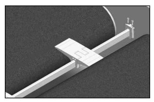
**9.** Slide the front plates on the mounting bar and replace the shims on top of the back plate. Then set the transfer into position on the back plates. Tighten the two socket head screws at each mounting bracket to secure the system in place.
