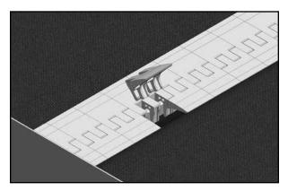
13. Install the last (trimmed) segments into the remaining gap. If the support bar does not appear centered in the gap between pulleys, loosen the socket head screws and adjust the transfer. 1/8" (3 mm) total adjustment is available.
