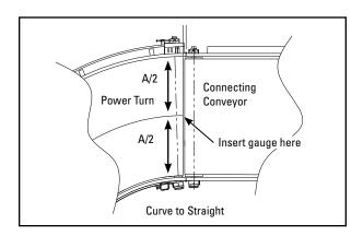
When inserting the STP gauge key, you should have a minimum distance between the top of the STP profile and the tangent point of the belt and the pulley of no less than  $\frac{1}{2}$ " (13 mm) for smaller diameter pulleys. For large diameter pulleys, the distance should not exceed 1-1/2" (38 mm). The bottom corner of the transfer plate plastic segment should have full contact with the belt and the key should rest level to the imaginary line that joins the crowns of the pulleys.
