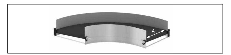
Once you have determined Dimension "A" (overall width of the conveyor), select the STP gauge key that properly fits in between the pulley where the transfer plate will be installed.
