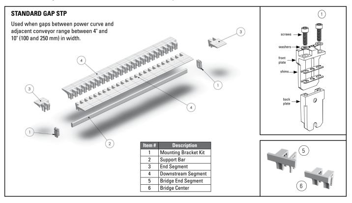
Flexco Segmented Transfer Plates are designed to absorb the damage of a foreign object and protect the belt from any injury while maintaining product flow. The transfer plate was designed to be compatible with polybags, nylon bags, small packages, and general parcel and material.
