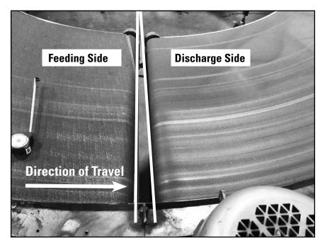
This is a typical example of a misaligned non friction driven conveyor system with two power curvesback-to-back. The gap between them narrows toward the inside of the power curve and widens toward the outside of the conveyor.
