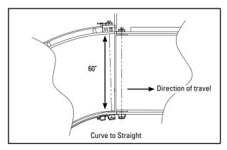
**6.** Position the support bar with segments and mounting brackets into the transfer gap. The resting position of the bar and the brackets should be similar to the one identified by the STP KEY location in SECTION 3. Ensure segments are not resting on top of the pulley crown or in the tapered section.
