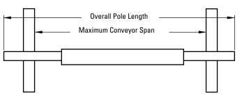
Pole Length Cleaner size + 1350mm Maximum Conveyor Span Cleaner size + 1100mm
