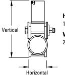
**Horizontal Clearance Required** 125mm
