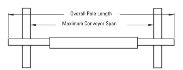
Pole Length Cleaner size + 1350mm (54") Maximum Conveyor Span Cleaner size + 1100mm (44")
