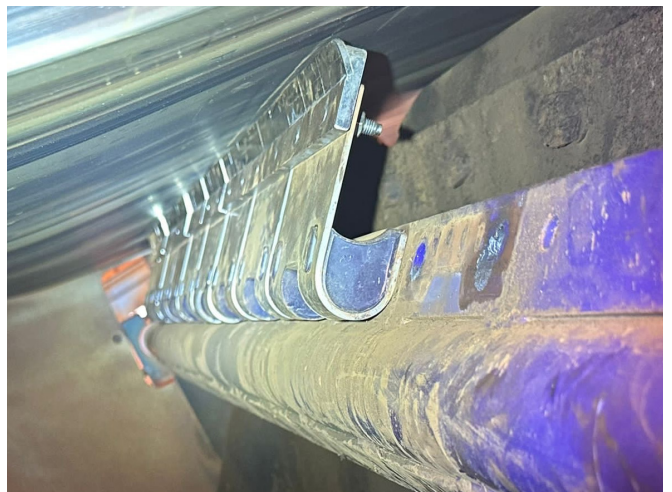
Shown: P-Type® Secondary Cleaner with Flextreme™ cushions
