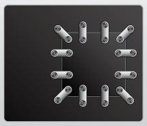
Larger size holes can be effectively repaired by applying standard Flexco® solid plate fasteners and a patch of belting as shown.
