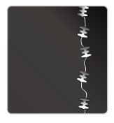
For quick temporary repairs, hammer-applied Turtle (TM) No.16 fasteners are recommended every four to six inches (101 to 152 mm) along the rip.
