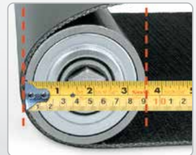
Measure smallest pulley diameter.
