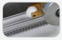
Clipper<sup>®</sup> maintenance lacers quick, on-site installation of G Series<sup>™</sup> lacing with precision Roller Lacing Technology<sup>™</sup>
