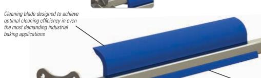
Simple to adjust spring tensioning unit ensures for maximum cleaning benefits Simple snap-in-place blade design allows for easy disassembly in less than a minute — no mechanical fasteners used in the product flow and no need to remove cleaner from structure for cleaning or replacement. Reassembly is just as quick so your line is up and running again fast
