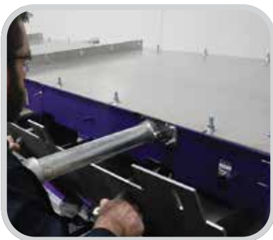
Externally replaceable liners for easy maintenance
