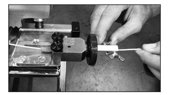
**3.** <u>Hand tighten</u> 2 wing screws on end block (M5 thread). Pull wire taut on tensioning end and ensure wire is located between fastener holes. <u>Hand tighten</u> remaining 2 wing screws.
