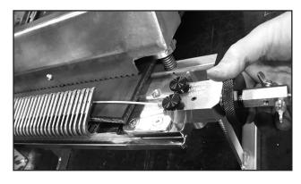
**4.** <u>Hand tighten</u> wire by turning tensioning knob clockwise until it becomes difficult to turn. Start fastener installation. Monitor wire tension and position during installation. Adjust if necessary. **Warning: Do not drive applicator over end block.**
