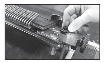
1. Load XP™ Staple Fasteners in bed starting on right side. Leave one empty slot. Center belt in fasteners and tighten clamp bar. Unscrew the 2 Phillips head plastic end screws on right side of frame and discard. Mount tensioning block using 2 black thumb screws (M6 thread). Hand tighten only.
