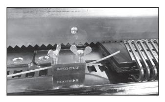
2. Position U-shaped end block approximately 2 slots from left edge of the belt. Secure from underneath with black thumb screw (M5 thread). <u>Hand tighten</u> only. Insert XP-LOK™ Belt Wire through blocks on both ends of the bed between belt and fastener. Leave minimum of 5 cm (50 mm) of excess wire on each end.
