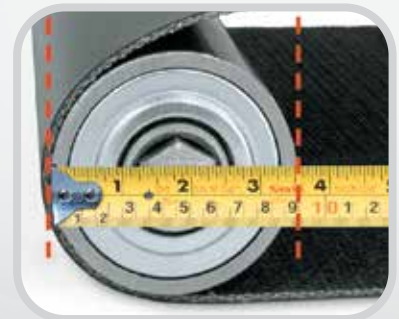
Measure smallest pulley diameter.
