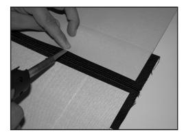
10. Using a soldering iron, fix ASL into belt at this position, fusing belt inner-layer to adhesive-primer on ASL. Belt end should follow stitch line across belt width, assuring a square splice. Sufficient fusing is required so that ASL does not disengage from belt during subsequent processing.
