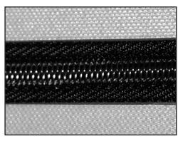
15. On the bottom side, belt inner-layer should melt, flowing slightly past belt ends, but not reaching spiral loops.
