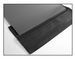
1. Cut belt ends square, yielding a belt length approximately 0.6" (15 mm) shorter than required finished length. Cut ASL to a length that is approximately 1.0" (25 mm) wider than belt width.
