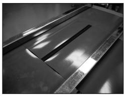
12. Place 3 mm silicone pad onto lower platen of  $Aero^{\infty}$  press. Trim ASL ends to be flush with belt edges. Place prepared ASL splice, conveying side upwards, onto 3 mm silicone pad. Fix belt in this position using Aero Belt Clamps. Fill balance of press width with belting.
