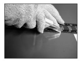
16. Remove belt from Aero $^{\infty}$  press. Use pliers to remove metal pin from ASL. Using carpenters square and knife, remove excess belt material, yielding straight belt edges.
