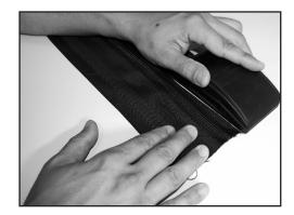
2. Using a Sanding Block / Sandpaper, lightly buff top and bottom surfaces of the fabric, raising a nap to improve mechanical bonding.
