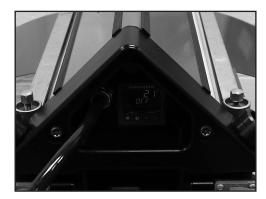
13. Place 0.5 mm silicone cloth (or silicone matrix pad) on top of prepared splice. Install Aero $^{\circ}$  Press upper beam, attaching it to lower beam using connecting bolts.
