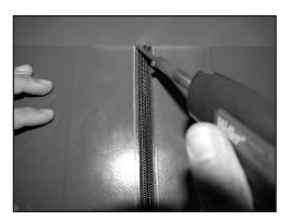
17. Use side-cutting pliers to remove a single spiral loop from outside edges of ASL. This will help prevent spiral loop from catching conveyor frame. Using soldering iron, cauterize ASL fabric at each belt edge to prevent fraying. Install plastic hinge pin.
