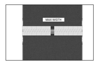
11. From the center of the bar, push the segment pairs toward the ends of the bar, ensuring that they are tightly butted against each other. Measure the gap that remains between the center-most segments to determine the size of the final segment set.
