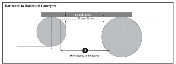
Dimension "B" will be obtained by locating a straight edge between the center lines of the pulleys. The dimension will be obtained by offsetting a parallel line towards the center of the pulley. The total offset should be between 13 mm to 38 mm below a line between the tangent points on the pulleys for most applications. The "B" dimension should be obtained by measuring the distance between the pulleys where the offset line intersects the outside diameter of the pulleys.
