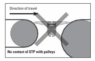
**WARNING:** This is an example of an incorrect installation. The transfer plate has no contact between the pulley and the plastic STP segments. Thin flat items and polybags will get caught in the gap and interfere with flow of material.
