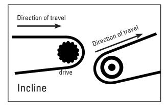
**2. Horizontal to Incline Conveyors.** Both conveyors are aligned and the belts have the same direction of travel. The first belt will feed the second belt. The second belt will have an upward direction.
