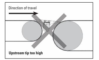
**WARNING:** This is an example of an incorrect installation. The transfer plate is installed above the head pulley and tilted downstream, this will create interference with the flow of material between the conveyors.
