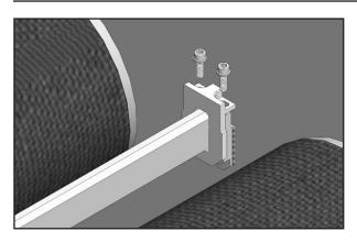
7. After verification that the tack weld has occurred, remove the socket head screws from the mounting brackets and lift the assembly with the front plates out of the transfer leaving only the back plates in place and finish welding the back plates with a 25 mm bead on two sides of the plate.
