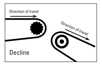
**3. Horizontal to Decline Conveyors.** Both conveyors are aligned and the belts have the same direction of travel. The first belt will feed the second belt. The second belt will have a downward direction.
