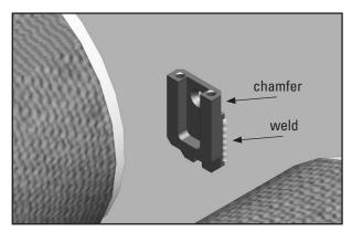
**6.** Welding instructions: With the assembly in place, tack weld the back plate onto the structure. Verify location after tack weld and adjust as needed.
