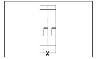
**CAUTION:** Do not trim more than half off a segment pair or 38 mm. It is recommended to trim both segments of a segment pair while they are nested to ensure consistent segment.
