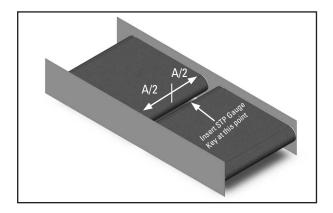
When inserting the STP gauge key, you should have a minimum distance between the top of the STP profile and the tangent point of the belt and the pulley of no less than 12.5 mm in smaller diameter pulleys. For large diameter pulleys, the distance should not exceed 38 mm. The bottom corner of the transfer plate plastic segment should have full contact with the belt and the key should rest level to the imaginary line that joins the crowns of the pulleys.
