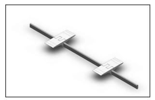
**2.** Slide one segment pair onto the bar from each end and position each approximately 6.35 mm of the total bar length from the end so that they do not rest on the top of the pulley crown or on the tapered section.
