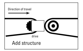
• In the particular case of waterfall conveyor arrangements (incline or decline configurations) there may be gaps where the conveyors meet. Make sure there is adequate structure to mount the transfer plate mounting brackets at the point of installation. If necessary, add a support plate to ensure safe and proper installation of the Segmented Transfer Plate mounting brackets.
