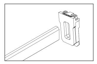
**4.** Slide one mounting bracket assembly onto each end of the bar. Ensure that the front plate is located in the center of the back plate slot to allow for maximum STP adjustment.
