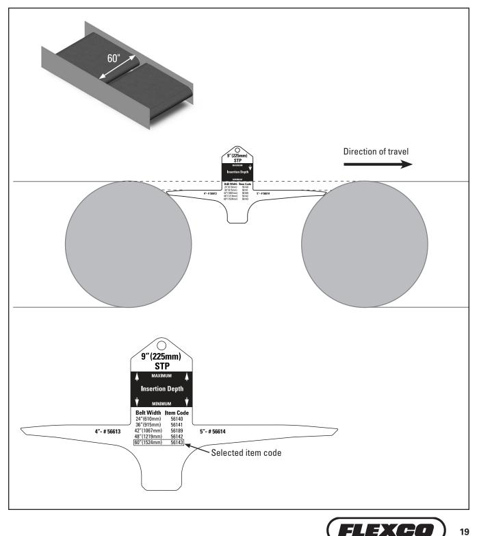
**IMPORTANT NOTE:** In the event that the segment transfer plate requires an offset installation, make sure the short segment is installed upstream (towards the head pulley or against the direction of travel). The downstream plastic segment (long segment) should be installed towards the trailing pulley (direction of travel).
