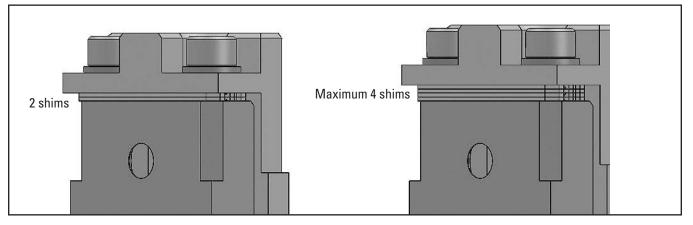
**13.** By adding or removing shims from the mounting brackets, the transfer can be adjusted up or down a total of 3 mm. This should allow adequate adjustment for crowned pulleys or a belt with a profiled top cover.
