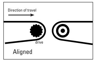
**1. Horizontal to Horizontal Conveyors.** Both conveyors are aligned and the belts have the same direction of travel. This arrangement is usually level.
