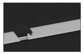
**9.** Install the remaining segments of the transfer plate, starting with the end segments.
