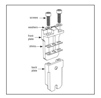
**3.** Stack two shims on top of back plate of each mounting bracket. Using socket head screws and washers, attach front plate to the back plate, ensuring that the shims are in place. Align the edges of the front and back plates so that the vertical edges are parallel. Tighten screws to compress shims, ensuring no interference with the pole end.
