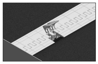
**12.** Install the last (trimmed) segments into the remaining gap. If the support bar does not appear centered in the gap between pulleys, loosen the socket head screws and adjust the transfer. 3 mm total adjustment is available.
