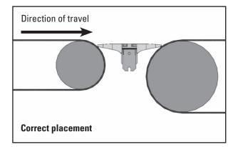
**Correct STP placement:** This is an example of a correct installation. The transfer plate is installed properly with adequate contact between the belt and the STP plastic segments.
