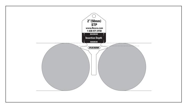
Incorrect placement of the STP Gauge Key, as described in the following examples, could lead to incorrect STP selection.
