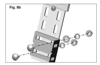
**8.** Determine desired position of the angle bracket (Fig. 8a). Use two bolts to loosely assemble angle bracket to vertical support at centre of desired slot location (Fig. 8b).
