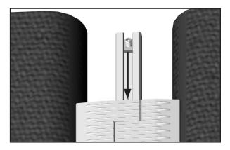
**Installation Hint:**Slide square nut and set screw until full contact with plastic segment.
