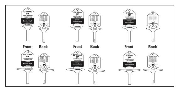
Determining the correct transfer plate item number and its location is a process of trial and error. We recommend that you prepare for the measurement process with an STP gauge key and measure the gap between the pulley until you achieve the correct fit between the STP gauge key and the pulleys. The following example will explain you the proper way to use the STP gauge key and how to select the correct Narrow Gap Segmented Transfer Plate item code for ordering.
