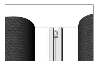
**18.** If the side structure is open and the extruded aluminum bar is cut longer than the inside wall of the conveyor structure, use included square nut and set screw to fix segments at both ends in place. This will prevent segment migration.
