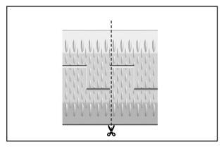
**CAUTION:** Do not trim more than half off a segment pair or 38 mm (1-1/2") off a segment pair. It is recommended to trim both segments of a segment pair while they are nested to ensure consistent segment.
