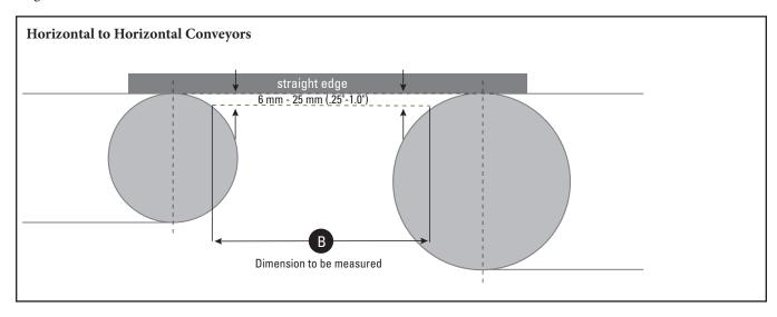
Dimension "B" will be obtained by locating a straight edge between the centre lines of the pulleys. The dimension will be obtained by offsetting a parallel line towards the centre of the pulley. The total offset should be between 6 mm (1/4") for small pulleys to 25 mm (1") for larger pulleys below a line between the tangent points on the pulleys. "B" dimension should be obtained by measuring the distance between the pulleys where the offset line intersects the outside diameter of the pulleys.
