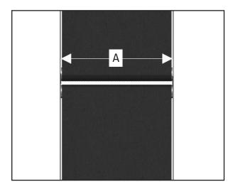
2. Measure the inside of the structure in order to determine the length of the transfer plate (Dimension A) at the point of the desired installation. This measurement will be required to properly select the transfer plate length and adequately install the plastic segments of the transfer plate.
