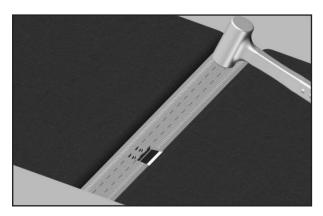
**17.** Install the last (trimmed) segments into the remaining gap.
