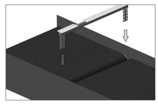
7. Place Segmented Transfer Plate into transfer opening.
