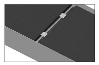
**3.** Slide one segment pair onto the bar from each end and position each approximately 6 mm (1/4) of the total bar length from the end. If your kit comes preassembled, please proceed to the next step.
