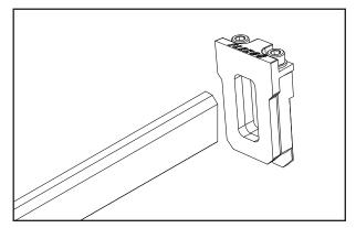
**4.** Slide one mounting bracket assembly onto each end of the bar. Ensure that the front plate is located in the centre of the back plate slot to allow for maximum STP adjustment.
