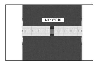
11. From the centre of the bar, push the segment pairs toward the ends of the bar, ensuring that they are tightly butted against each other. Measure the gap that remains between the centre-most segments to determine the size of the final segment set.
