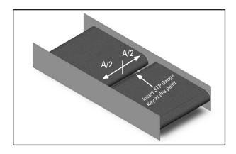
When inserting the STP gauge key, you should have a minimum distance between the top of the STP profile and the tangent point of the belt and the pulley of no less than 12.5 mm ( $\frac{1}{2}$ ) in smaller diameter pulleys. For large diameter pulleys, the distance should not exceed 38 mm (1.5"). The bottom corner of the transfer plate plastic segment should have full contact with the belt and the key should rest level to the imaginary line that joins the crowns of the pulleys.
