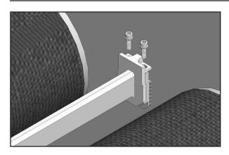
7. After verification that the tack weld has occurred, remove the socket head screws from the mounting brackets and lift the assembly with the front plates out of the transfer leaving only the back plates in place and finish welding the back plates with a 25 mm (1") bead on two sides of the plate.
