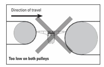
**WARNING:** This is an example of an incorrect installation. The transfer plate is installed below the correct placement position, it will cause the flow of material to choke between the conveyors.
