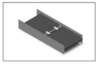
**5.** Position the support bar with segments and mounting brackets into the transfer gap. The resting positon of the bar and the brackets should be similar to the one identified by the STP KEY location in SECTION 3. Ensure segments are not resting on top of the pulley crown or in the tapered section.
