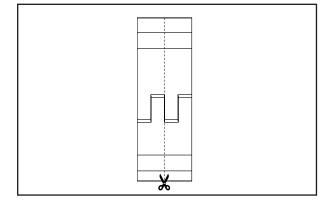
**CAUTION:** Do not trim more than half off a segment pair or 38 mm (1.5"). It is recommended to trim both segments of a segment pair while they are nested to ensure consistent segment.
