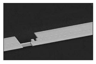
**9.** Install the remaining segments of the transfer plate, starting with the end segments.
