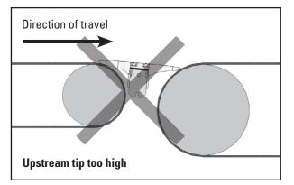
**WARNING:** This is an example of an incorrect installation. The transfer plate is installed above the head pulley and tilted downstream, this will create interference with the flow of material between the conveyors.
