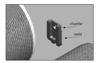
**6.** Welding instructions: With the assembly in place, tack weld the back plate onto the structure. Verify location after tack weld and adjust as needed.
