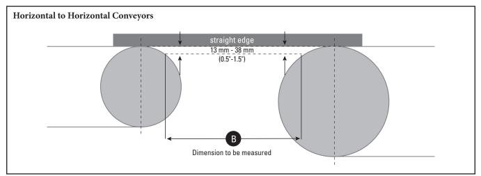
Dimension "B" will be obtained by locating a straight edge between the centre lines of the pulleys. The dimension will be obtained by offsetting a parallel line towards the centre of the pulley. The total offset should be between 1/2" (13 mm) to 1.5" (38 mm) below a line between the tangent points on the pulleys for most applications. The "B" dimension should be obtained by measuring the distance between the pulleys where the offset line intersects the outside diameter of the pulleys.
