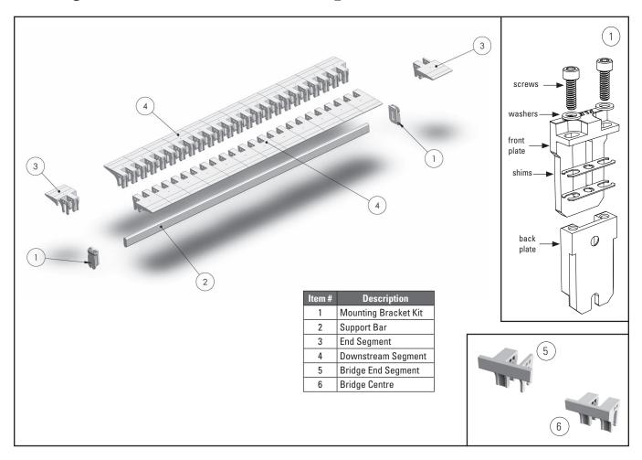
Flexco Segmented Transfer Plates are designed to absorb the damage of a foreign object and protect the belt from any injury while maintaining product flow. The transfer plate was designed to be compatible with polybags, nylon bags, small packages, and general parcel and material.
