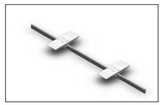
**2.** Slide one segment pair onto the bar from each end and position each approximately 1/4 of the total bar length from the end so that they do not rest on the top of the pulley crown or on the tapered section.
