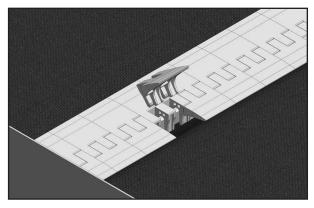
**12.** Install the last (trimmed) segments into the remaining gap. If the support bar does not appear centred in the gap between pulleys, loosen the socket head screws and adjust the transfer. 3 mm (1/8th inch) total adjustment is available.
