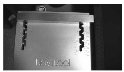
Lock adjusting guide to 120 mm.
