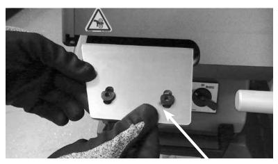
Remove blade carefully. Remove blade nuts and set aside for future use. Retain brass spacers should they release with the bolts.
