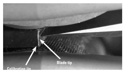
Apply pressure to the back side of blade so that the blade tip squarely rests against the calibration jig.
