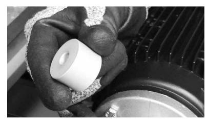
After removal of torque arm bolt set spacer aside.
