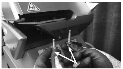
Ensure brass spacers are present either in the Ply frame or on bolt. Finger tighten bolts only so that the blade can still shift (long bolt in rear and short bolt in front).
