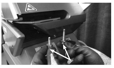
Ensure brass spacers are present either in the Ply frame or on bolt. Finger tighten bolts only so that the blade can still shift (long bolt in rear and short bolt in front).
