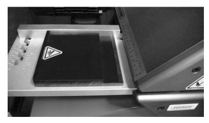
Place calibration jig on feed table with thin edge toward rollers. Plug in power connection. Turn switch to 'FORWARD'.
