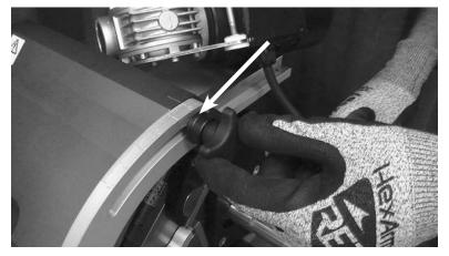
Position and lock adjusting handle so that adjusting screws are accessible.
