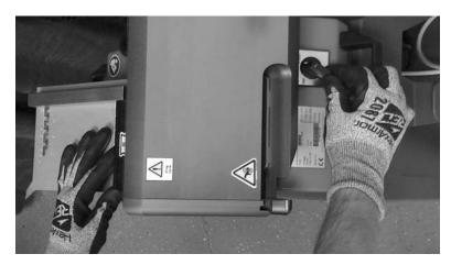
Reconnect power cable to electrical power supply. Rotate switch to 'REVERSE' to release calibration jig from between traction rollers.
