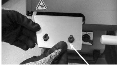
Remove blade carefully. Remove blade nuts and set aside for future use. Retain brass spacers should they release with the bolts. **Warning:** Do not touch blade edge.
