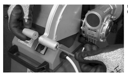
Using a 5 mm hex key, remove the handle.
