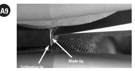
Apply pressure to the back side of blade so that the blade tip squarely rests against the calibration jig.
