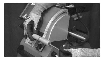
Once adjustments have been made, reinstall the guard plate. Start by reinstalling the handle.
