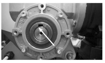
For easier removal of motor ensure keyway is positioned at top of drive shaft.
