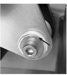
**ote:** Ensure rubber grommet is in place ior to reassembly.
