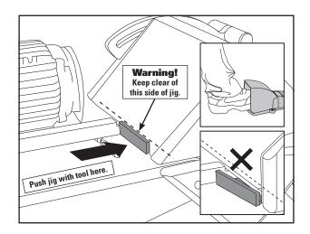
With moderate force, push calibration jig into Ply 130 using a block of wood or tool simultaneously turning on Ply with foot switch. When lip of jig is tight up against the Ply frame, release the foot switch and toggle operating switch to "OFF". Disconnect power.
