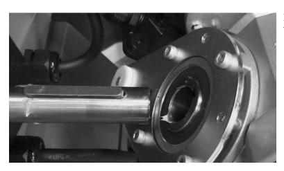
Reinstall motor. Align shaft key with key slot.
