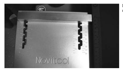
Lock adjusting guide to 120 mm.
