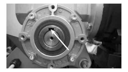
For easier removal of motor ensure keyway is positioned at top of drive shaft.
