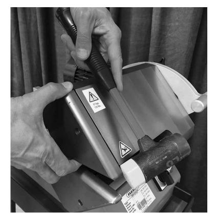
Lightly tap at back edge of top faceplate with a rubber mallet until a small opening appears in between the top cover plate and the Ply 130 body. A small rubber tipped chisel may be required if the faceplate is a tight fit.
