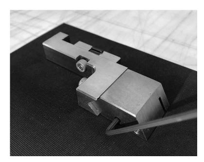
Loosen blade retention setscrews using 2.5 mm hex wrench. Do not loosen the flat head screw on opposite side.
