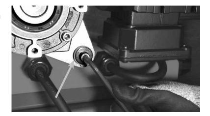
Remove the electric motor to gain sufficient access for adjustment of traction rollers by first removing the torque arm bolt using a 6 mm hex wrench.
