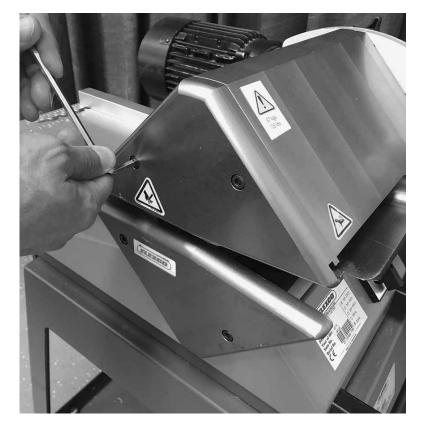
Using a hex key, tightly secure the two 5 mm hex screws adhering faceplate to Ply 130 frame.
