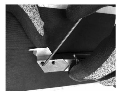
Carefully insert step cutting blade into position, aligning edge of blade even with step cutter face to ensure proper blade position. Tighten blade retention setscrews.
