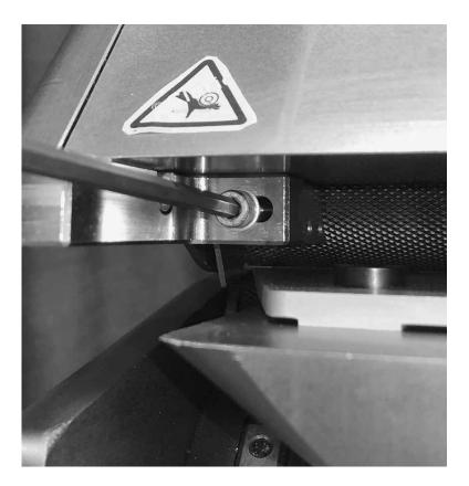
If necessary, use the 2.5 mm hex key to loosen screw and adjust lateral position of step-cutting blade up to ply separation blade. Tighten screw to fix blade position. If ply separation blade is replaced (refer to Ply 130™ Safety and Operations Manual for instructions) confirm the lateral adjustment position of step cutting blade. If necessary, use the 2.5 mm hex key to loosen screw and then laterally adjust the step cut blade up to the new ply separation blade.
