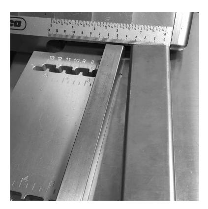
Install Guide Extension for step cutting less than 1.57" (40 mm). Loosen infeed table clamp nuts. Lift adjustable guide and insert guide extension under adjustable guide. Position guide to desired step cutting depth and tighten clamp nuts.
