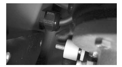
Reassemble the motor to the frame placing the spacer between the motor torque arm and ply base. Insert 8 mm hex bolt with washer and tighten.
