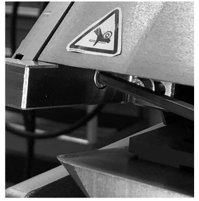
Using the T-handle hex key, tighten Step-Cutter T-nut screw.
