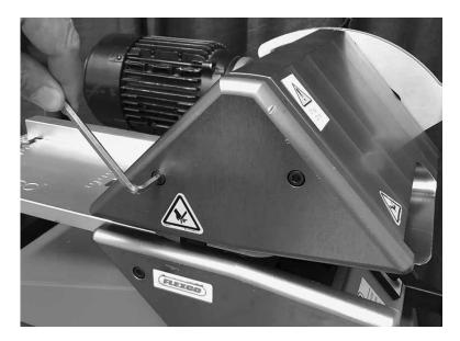
**Caution!** Disconnect Ply 130 plug from the power source. Remove the two 5 mm hex screws from existing top faceplate on Ply 130.
