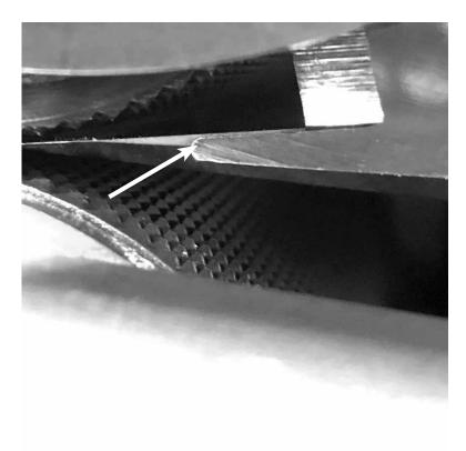
Step cutter blade leading guide needs to be flush with the top surface of the standard ply blade or slightly below.
