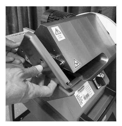
With fingerguard dowel pins properly aligned, mount Step Cutter faceplate flat to Ply 130 body, lightly tapping with plastic hammer if required.
