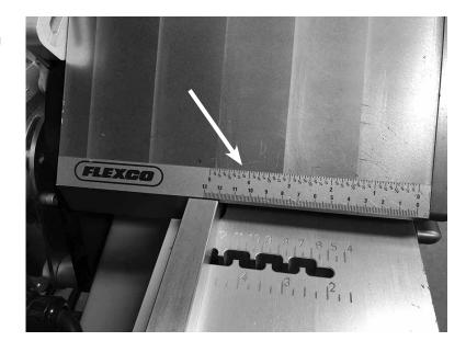
Clean top surface of Ply 130 body nearest to infeed table. Remove backing paper from scale decal and install on Ply 130 body. Align to edge of Ply Separator body.
