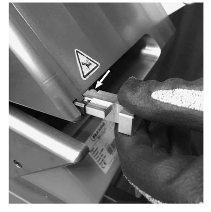
Loosen (do not remove) T-nut screw. Align step cutter T-nut with T-groove in faceplate.
