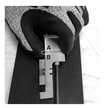
Ensure that the brass step cutter blade holder (A) is adjusted flush with the T-nut side (B) of the main fixture.
