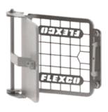
Chute Opening: 500 mm x 500 mm Outer Door: Solid c/w Lockable Handle Inner Mesh Door: 3 mm mesh @ 50 mm spacing Material: Grade 316 Stainless Steel Overall Weight: 18 kg
