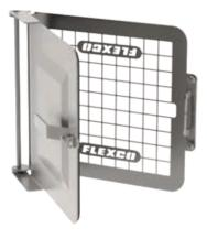
Chute Opening: 400 mm x 400 mm Outer Door: Solid c/w Lockable Handle Inner Mesh Door: 3 mm mesh @ 50 mm spacing Material: Grade 316 Stainless Steel Overall Weight: 13 kg
