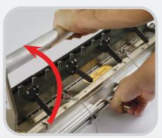
**Simple Adjustment:**After the fasteners are initially set, simply flip the handle.
