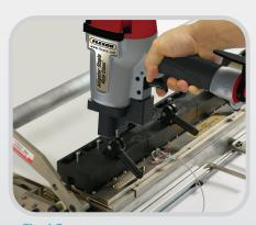
Final Set: With additional trigger pulls, the staples receive their final set and the compression fit is obtained.
