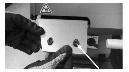
Remove blade carefully. Remove blade nuts and set aside for future use. Retain brass spacers should they release with the bolts.
