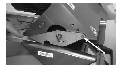
Reinstall finger guard ensuring that dowels are installed in the Ply 130 body as shown.
