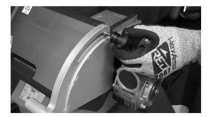
If adjustment is needed, unscrew clamp nut on adjustment guard plate.
