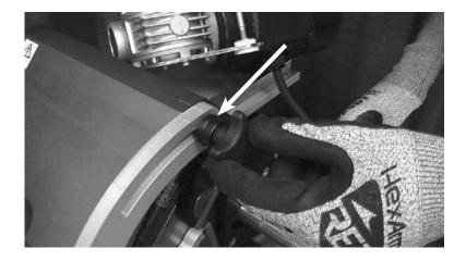
Position and lock adjusting handle so that adjusting screws are accessible.
