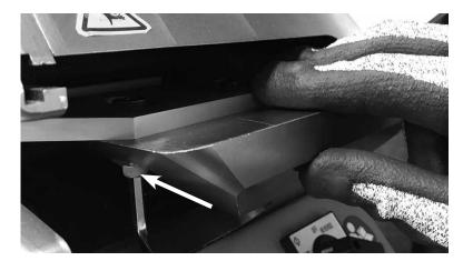
Tighten bolts firmly while keeping cutting edge of blade squared up against the jig.
