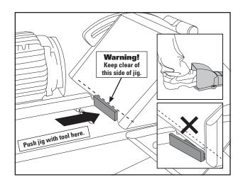
With moderate force, push calibration jig into Ply 130 using a block of wood or tool simultaneously turning on Ply with foot switch. When lip of jig is tight up against the Ply frame, release the foot switch and toggle operating switch to "OFF". Disconnect power.
