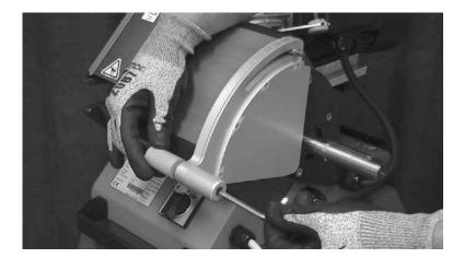
Once adjustments have been made, reinstall the guard plate. Start by reinstalling the handle.
