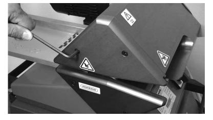
Using a hex key, tightly secure the two 5 mm hex screws securing faceplate to Ply 130 frame.
