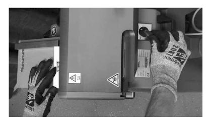
Reconnect power cable to electrical power supply. Toggle switch to 'REVERSE' to release calibration jig from between traction rollers.
