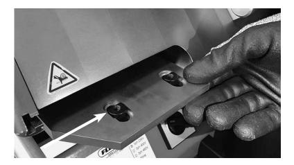
Insert nuts so that bevels are facing toward traction rollers.
