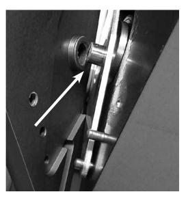
With traction roller and dowel pins properly aligned, mount faceplate flat to Ply 130 frame, lightly tapping with rubber mallet, if required.
