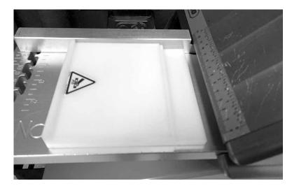
Place white calibration jig on feed table with thin edge toward rollers. Plug in power connection. Turn switch to 'FORWARD'.
