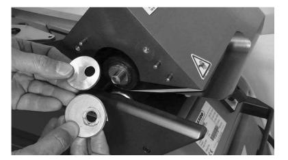
Replace brass spacer with smaller diameter spacer.
