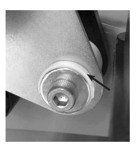
**Note:** Ensure rubber grommet is in place prior to reassembly.
