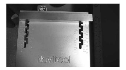
Lock adjusting guide to 120 mm.
