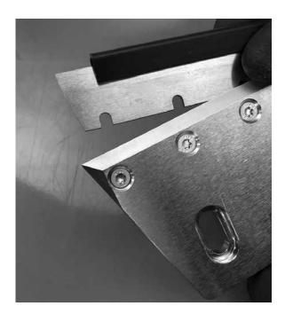
Keeping blade cover on, install blade insert bevel side down.
