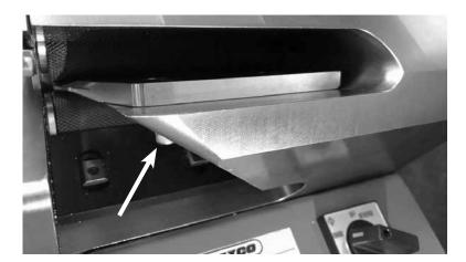
Tighten bolts firmly while keeping pressure of blade against the jig.
