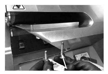
Ensure brass spacers are present either in the Ply frame or on bolt. Finger tighten bolts only so that the blade can still shift (long bolt in rear and short bolt in front).
