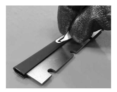
Remove safety decal from new blade insert.
