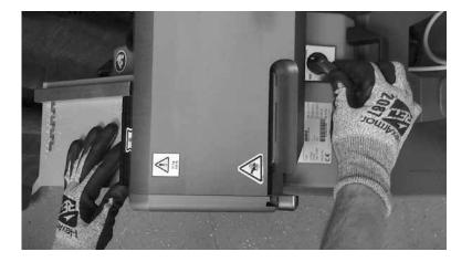
Reconnect power cable to electrical power supply. Rotate switch to 'REVERSE' to release calibration jig from between traction rollers.
