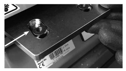
Insert blade nuts so that bevels are facing toward traction rollers.
