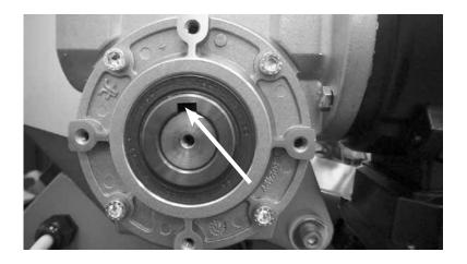
For easier removal of motor ensure keyway is positioned at top of drive shaft.
