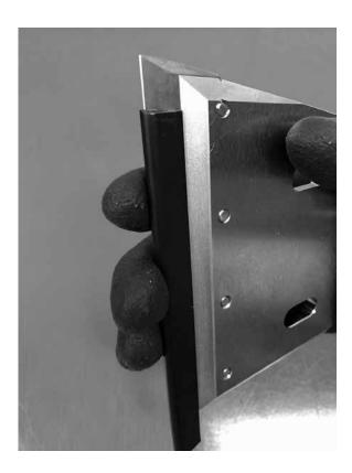
Underside view of blade holder with blade properly installed.
