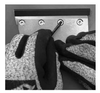
Securely tighten all four torx screws.
