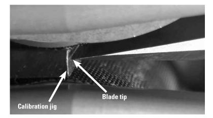
Apply pressure to the back side of blade so that the blade tip squarely rests against the calibration jig.
