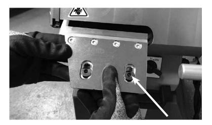
Remove blade carefully. Remove blade nuts and set aside for future use. Retain brass spacers should they release with the bolts.
