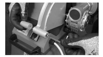
Using a 5 mm hex key, remove the handle.
