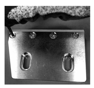
Position blade holder with the four countersunk holes up.
