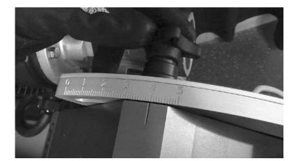
Lock adjusting handle in position 4.0 to 4.5.
