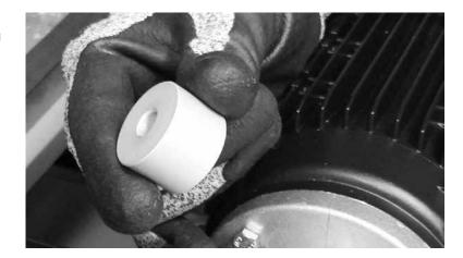
After removal of torque arm bolt set spacer aside.
