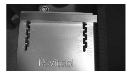
Lock adjusting guide to 120 mm.
