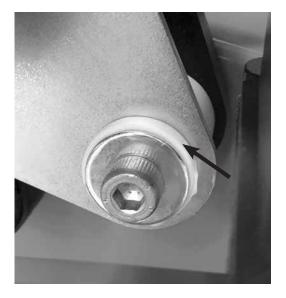
**Note:** Ensure rubber grommet is in place prior to reassembly.
