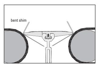
**Installation Hint:** In order for the shims to stay in place, you can bend them so that they will stay put while you maneuver the assembly into place.
