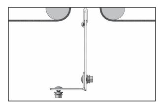
10. Position vertical support brackets so that the angle brackets are in position for final attachment to structure. Tighten the vertical support bracket to the extruded aluminum bar using the supplied button head screw. This will prevent extruded aluminum bar from migration.
