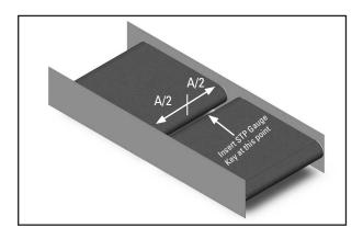
When inserting the STP gauge key, you should have a minimum distance between the top of the STP profile and the tangent point of the belt and the pulley of no less than 6.25 mm (1/4") in smaller diameter pulleys. For large diameter pulleys, the distance should not exceed 25 mm (1"). The bottom corner of the transfer plate plastic segment must have full contact with the belt and the key should rest level to the imaginary line that joins the crowns of the pulleys.
