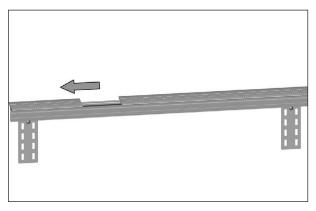
**6.** Slide two to three segment pairs down to the end of the extruded aluminum bar.
