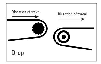
**4. Horizontal to Horizontal Drop Conveyors** Both conveyors are aligned, but not level and the belts have the same direction of travel. The first belt will feed the second belt. There is a clear drop between the belts.
