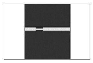
14. Install remaining segments until last gap remains. Gap will likely be smaller than segment width.
