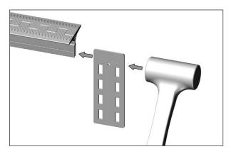
**4.** Insert vertical support mount into extruded support bar using light hammer taps (Fig 3). Position vertical support bracket in approximate final location, no further than 150 mm (6") from end (final location to be determined in Step 4.1.8).
