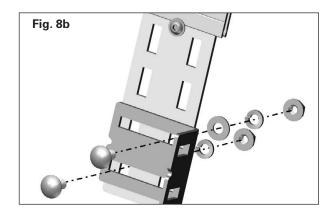
**8.** Determine desired position of the angle bracket (Fig. 8a). Use two bolts to loosely assemble angle bracket to vertical support at center of desired slot location (Fig. 8b).
