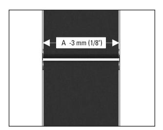
2. Installation hint: In the event that the bar does not pass the structure or if the bar and segments cannot pass through the side structure of conveyor, cut the support bar to the proper length: structure width minus 3 mm (1/8").
