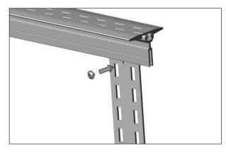
**5.** Use button head screw to lightly secure vertical support bracket to extruded support bar.
