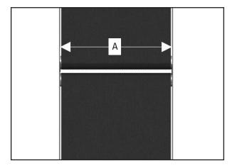
Once you have determined dimension "A" (overall width of the conveyor), select the STP gauge key that properly fits in between the pulley where the transfer plate will be installed.
