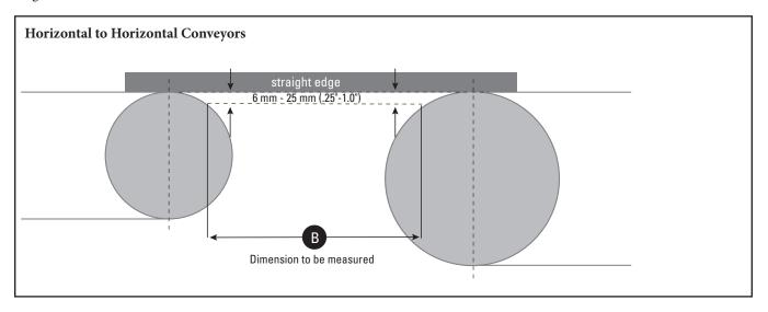
Dimension "B" will be obtained by locating a straight edge between the center lines of the pulleys. The dimension will be obtained by offsetting a parallel line towards the center of the pulley. The total offset should be between 6 mm (1/4") for small pulleys to 25 mm (1") for larger pulleys below a line between the tangent points on the pulleys. "B" dimension should be obtained by measuring the distance between the pulleys where the offset line intersects the outside diameter of the pulleys.
