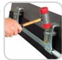
Quick adjustment by using the locking wedges on the clamp pins
