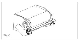
**5.** Test fit cleaner without blade. Pole should be parallel to the pulley (Fig. C).
