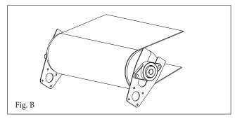
**4.** Temporarily mount 2nd bracket onto the opposite side of conveyor (Fig. B).
