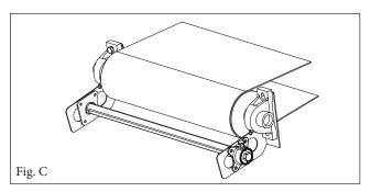
**5.** Test fit cleaner without blade. Pole should be parallel to the pulley (Fig. C).
