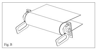
**4.** Temporarily mount 2nd bracket onto the opposite side of conveyor (Fig. B).
