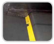
Segment released due to F.O.D (foreign object debris)
