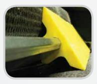
**Snap-fit design:** The 76 mm (3") segments are designed to release under pressure if small objects become lodged between belt and segments.
