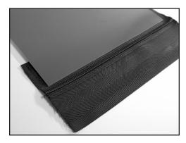
1. Cut belt ends square, yielding a belt length approximately 15 mm shorter than required finished length. Cut ASL to a length that is approximately 25 mm wider than belt width.
