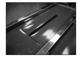
**12.** Place 3 mm silicone pad onto lower platen of Aero<sup> $\infty$ </sup> press. Trim ASL ends to be flush with belt edges. Place prepared ASL splice, conveying side upwards, onto 3 mm silicone pad. Fix belt in this position using Aero Belt Clamps. Fill balance of press width with belting.
