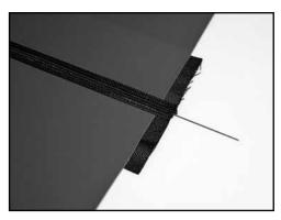
**11.** Insert a metal pin as a hinge pin, connecting the ASL spiral. Metal pin diameter should correspond with ASL type as indicated in the below chart. Pin should be minimally 100 mm longer than belt width.
