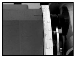
7. Using the Ply 130<sup>∞</sup>, prepare belt ends. Position the Ply 130 adjustment to separate between two fabric plies of the belt. Residual of plastic inner-layer must remain on each plastic ply. Separation should be near center-plane of all fabric plies.
