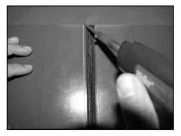
17. Use side-cutting pliers to remove a single spiral loop from outside edges of ASL. This will help prevent spiral loop from catching conveyor frame. Using soldering iron, cauterize ASL fabric at each belt edge to prevent fraying. Install plastic hinge pin.
