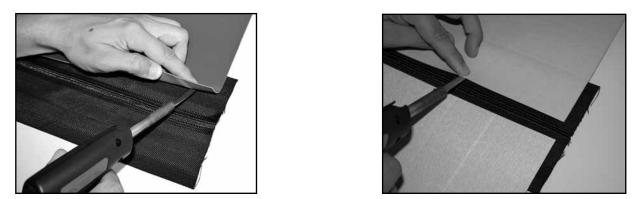
**10.** Using a soldering iron, fix ASL into belt at this position, fusing belt inner-layer to adhesive-primer on ASL. Belt end should follow stitch line across belt width, assuring a square splice. Sufficient fusing is required so that ASL does not disengage from belt during subsequent processing.
