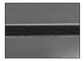
14. Fuse ASL into belt using Aero<sup>™</sup> Press. Splice parameters will be similar as with finger splicing. Belt inner-layer should melt, flowing slightly past belt ends, but not reaching spiral loops.
