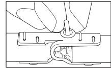
7. To keep rocker pins in place, push pin retainer through gap in top of fastener as shown.
