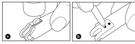
4. Lift holder off belt and remove the back staple.
