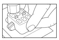
**3.** Push male or female half of fastener over belt and into recess in holder as far as it will go. Look into staple slot in holder and make sure holes in fastener are visible. Drive staple into belt flush with holder.
