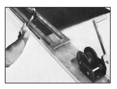
2. Lay a clear, (free of knots or nails) straight wooden plank, minimum 2" x 8", on a firm surface crosswise under the belt and under squared line. Nail winch on one end. Be sure winch handle operates freely. Nail track along squared line or square edge of belt (use every hole on both sides of track over belt) with opening for skiver head at opposite end from winch. Use No. 16D coated nails provided. Reset all nails.
