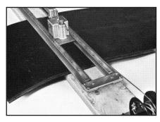
**6.** Loosen blade-depth and lower blade until it contacts wood base. Connect winch cable to skiver head and crank it across. Silicone spray on belt will help. Retract blade and remove skiver head and track from belt. Repeat operation on opposite end of belt.
