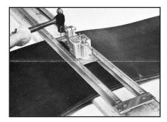
4. Hook winch cable on ½" bolt on top of skiver and crank winch to draw skiver across the belt. Spray Flexco® silicone lubricant on track and belt. After skiver cuts about six inches, stop and nail the skived flap back in place to keep flap from jamming in skiver. Complete the skive. Adjust skiver blade back up into skiver head and return skiver head to start position.
