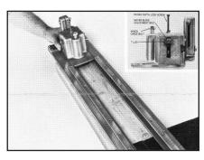
3. Warning: Skiver and cutter blades are unguarded and extremely sharp. On a woven belt, calculations for belt thickness should be made in center of belt. Set skiver blade by loosening bolts on either side of skiver head and aligning T-lug on 1/16" marks (these marks are approximate and may vary slightly due to belt cover hardness) for depth of cut. Retighten bolts and put skiving head on opening in track with skiver blade toward belt edge.
